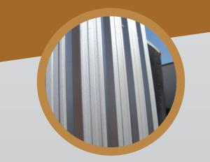
**Diamond Rib Reverse Application/Specifications** Use: Wall Coverage: 36" wide Length: 3' to 45' Rib Height: 3/4" reverse rib on 6" centres Fastener System: Exposed Fastener Recommended Substrate: Open Framing or Solid Substrate
