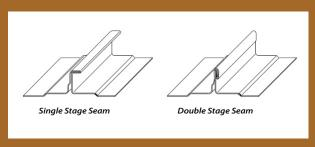
Standing seam panels can be seamed as a single stage seam or as a double stage seam, using a hand crimper or power seamer.
